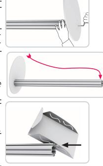
connector bars should be at column. Grooves containing Attach base plate to lower
