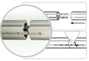
assembly secure. Repeat Join posts and tighten for other base post.
